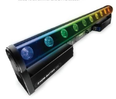
The Show Batten lens is fitted with a wide electronic linear zoom. The "Show Batten AS" version has a special ovalizer filter instead of the standard lens, which increases the projection angle on a single axis. This is particularly suitable for wall washing. The zoom is very fast: 0.3 s from min. to max.
