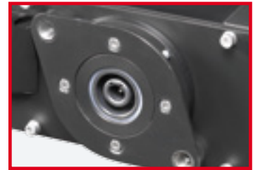
Bayonet connector for battery charging using the special flight case
