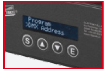
black and white backlit 2x16 characters LCD display
