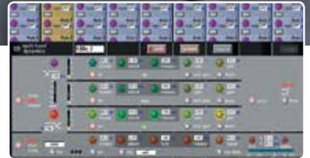
> Multi-band compression is perfect for use with in ear monitor mixes, keeping the artist safe from damaging high frequencies or just smoothing out the tonal balance of the mix simply and effectively allowing you to concentrate on mixing the show.
